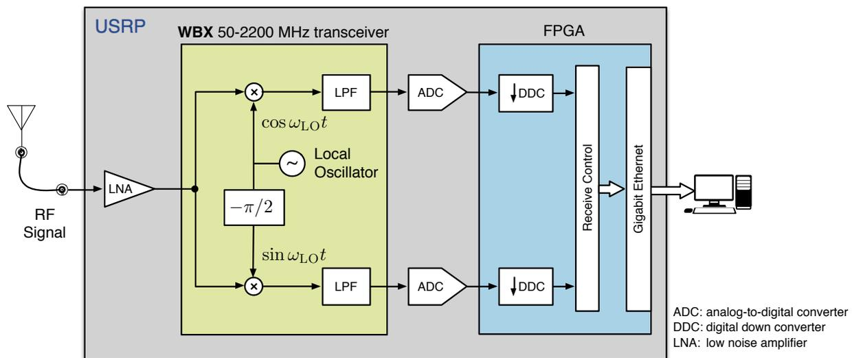
**Figure 3:** Receiver subsystem of Ettus Research N210 USRP.
