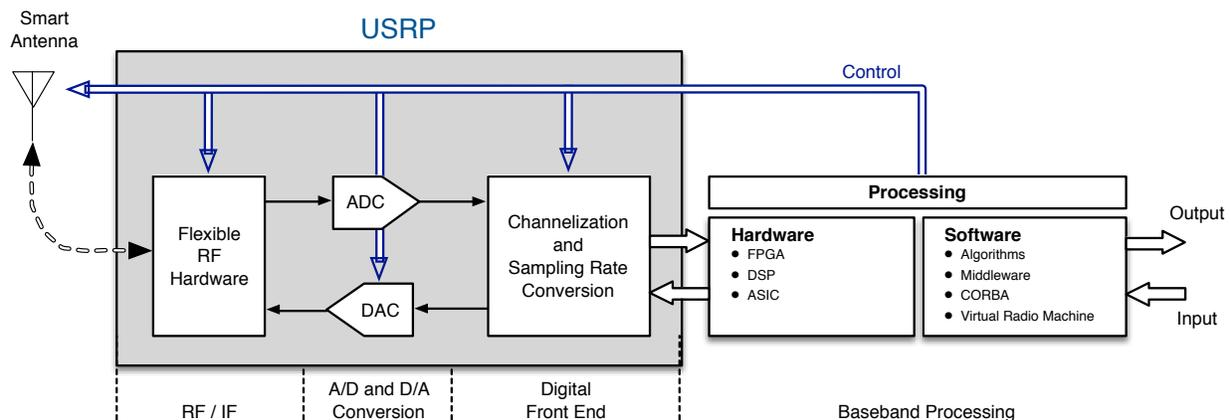
**Figure 1:** Basic SDR architecture [1].
