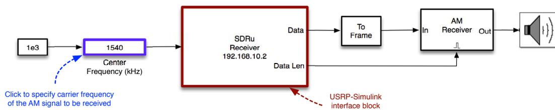
**Figure 4:** AM Receiver top-level signal flow diagram.
