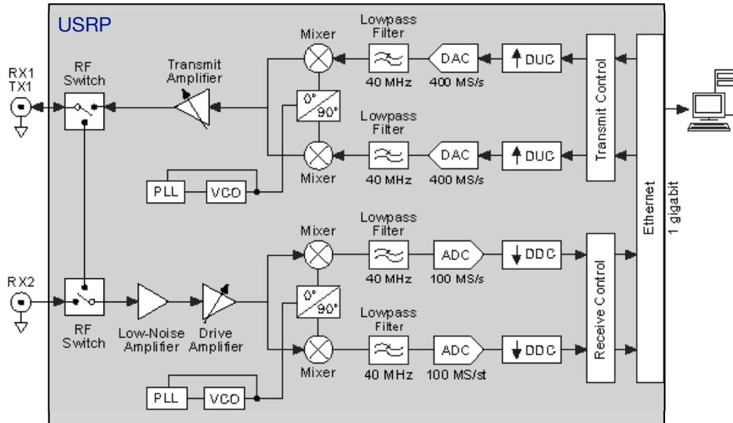
**Figure 2:** N210 USRP architecture with WBX wide bandwidth transceiver card [2].
